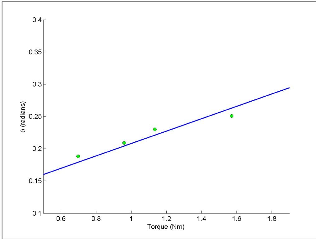
**Figure 4** Linear regression of torque vs. angle data
