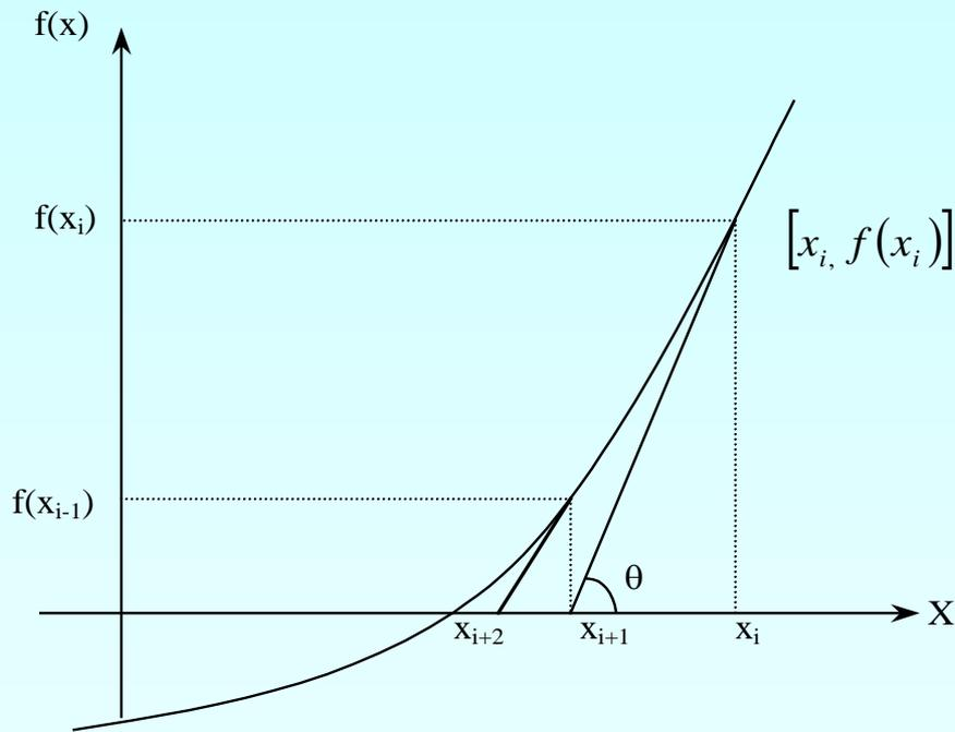
**Figure 1** Geometrical illustration of the Newton-Raphson method.
