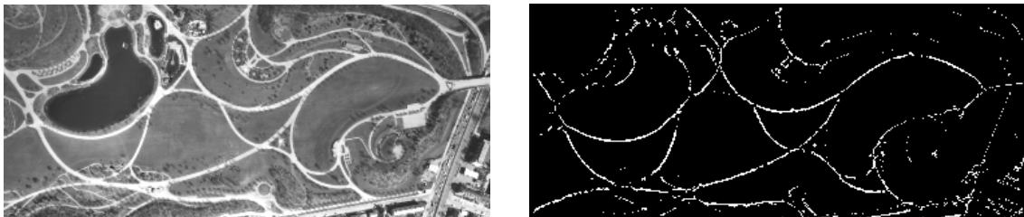
Figure 1 On left is an aerial image of park in Munich, Germany. We see the roads and a lake. On the right is the road network extracted from the image.
