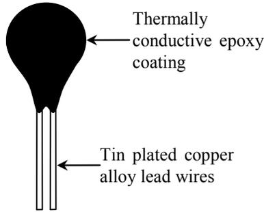
**Figure 5** A typical thermistor.
