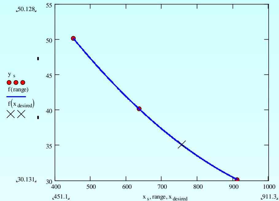
$$T(R) = b_0 + b_1(R - R_0) + b_2(R - R_0)(R - R_1)$$
