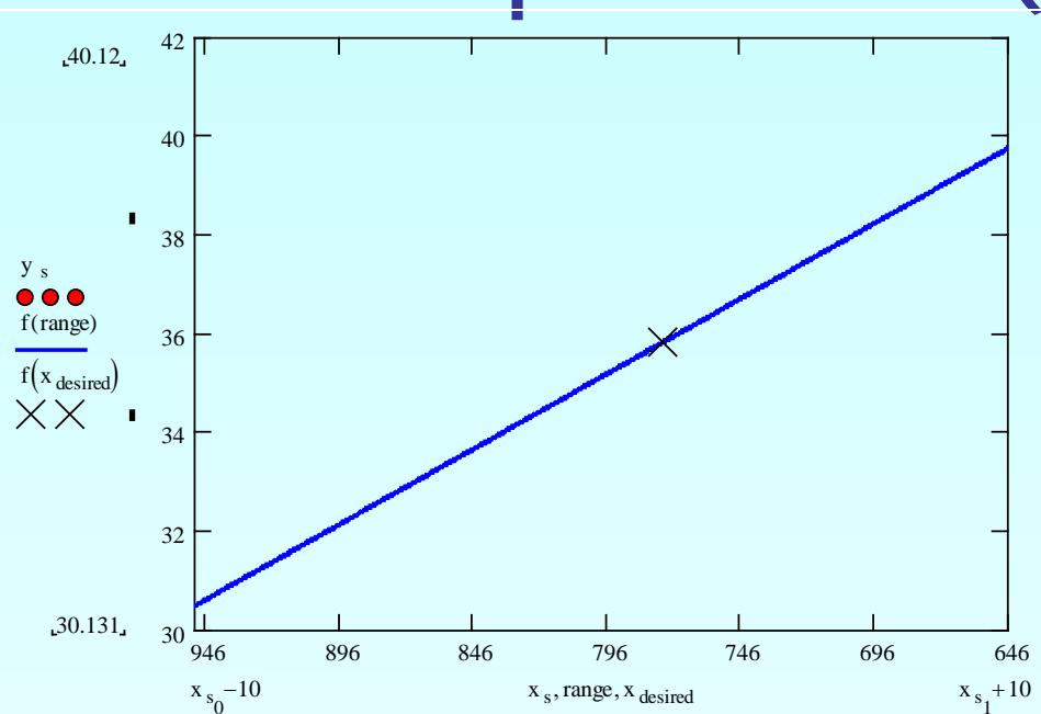
$$\begin{aligned}T(R) &= b_0 + b_1(R - R_0) \\&= 30.131 - 0.036284(R - 911.3), \quad 636.0 \leq R \leq 911.3\end{aligned}$$
