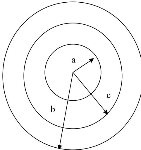
**Figure 2** A compounded cylinder pressure vessel with internal radius,  $a$ , outer radius,  $b$ , and interface at  $r = c$ .
