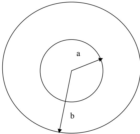
**Figure 1** A single cylinder pressure vessel with internal radius,  $a$  and outer radius,  $b$ .
