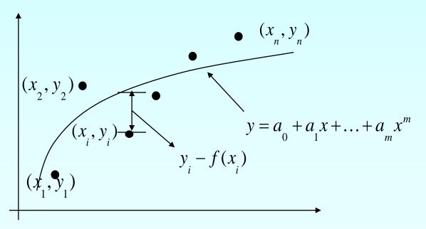
Figure. Polynomial model for nonlinear regression of y vs. x data
