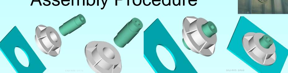
**Step1**. Trunnion immersed in dry-ice/alcohol
