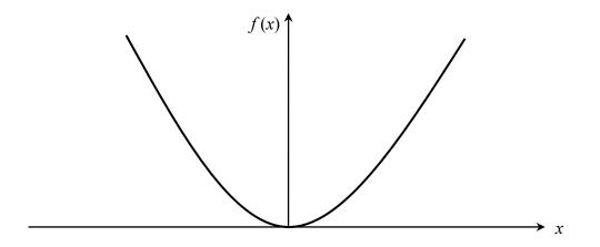
Figure 6 The equation  $f(x) = x^2 = 0$  has a single root at x = 0 that cannot be bracketed.
