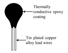
Figure 5 A typical thermistor.
