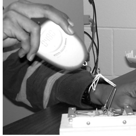
Figure 4. Twisting the mousetrap spring experiment
