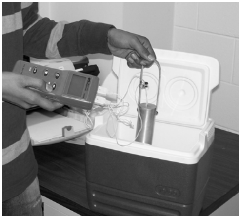
Figure 1. Immersing aluminum cylinder in iced-water experiment
